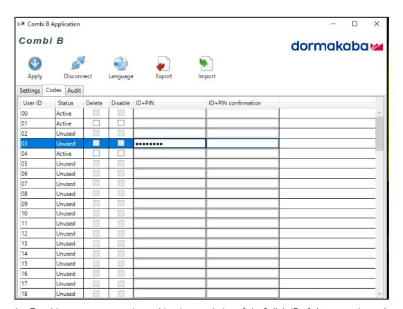
1. To add a user, enter a code combination consisting of the 2 digit ID of the respective code and 6 freely selectable digits.
