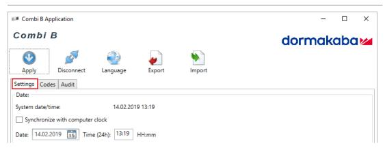
It is possible to transfer the current system time (date and time) or the manually set time to the lock.
