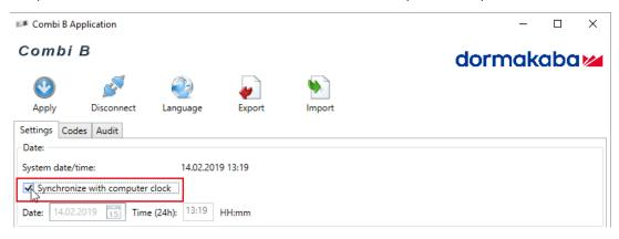
1. Select the checkbox 'Synchronize with the computer clock'.
